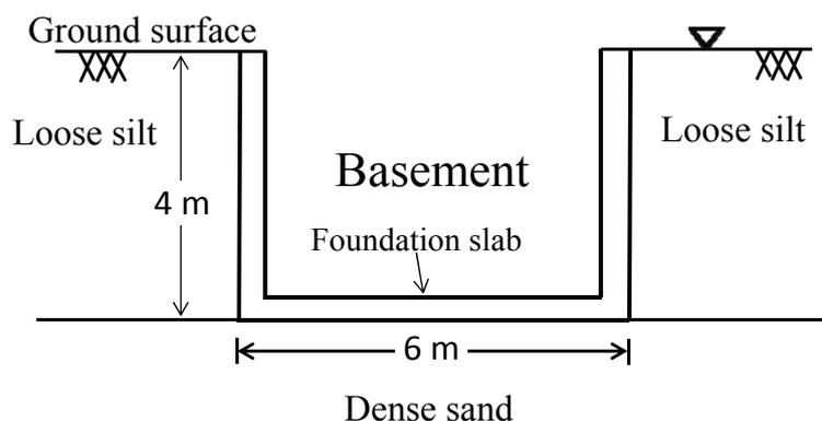
Q.52 Using factor of safety = 3, the net safe bearing capacity (in  $\text{kN/m}^2$ ) of the foundation is:
